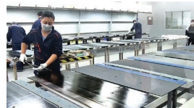
Skilled coating operators ensure each anode is coated to precise application requirements
